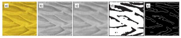
Figure 5. Image process of wrinkled fabric; a) coloured image, b) grey level image, c) median filtered image, d) binary image, e) edge detected image.
