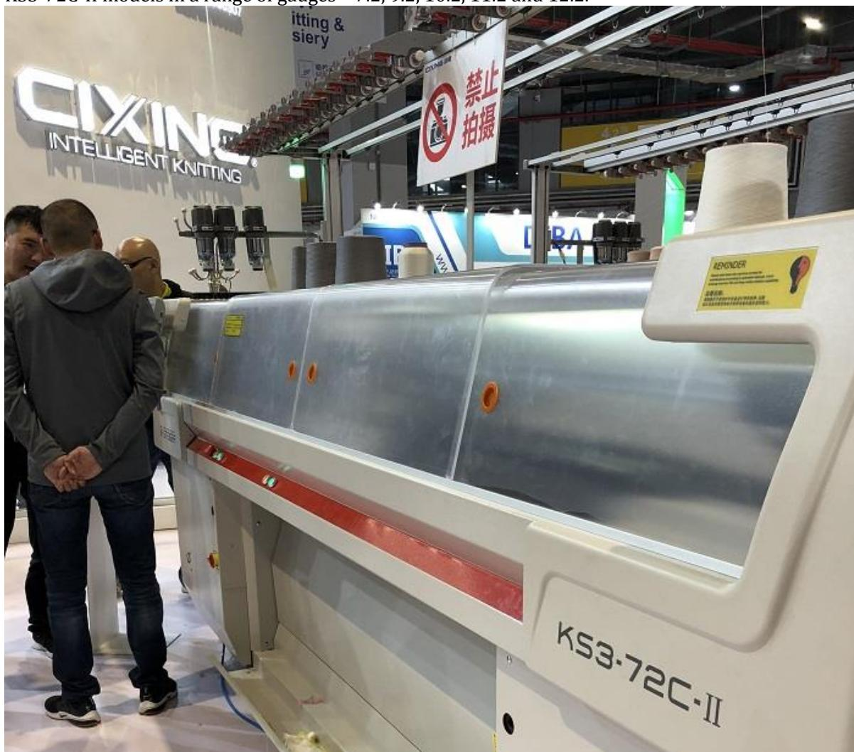
The KS3-72C is a brand-new range of complete garment knitting machines which Cixing staff and Cixing-Steiger product catalogues claim are actually four-needlebed machines. To date, only Japanese technology leader Shima Seiki has developed a four needlebed machine. According to Daniel Chen, a Regional Sales Manager at Cixing, who escorted me on a tour of the booth, the machines were definitely four needlebed machines with needles and selector jacks on all four needlebeds.
